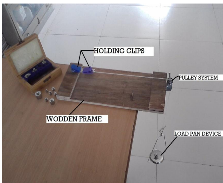
Figure 1: The tensiometer used to measure the tensile strength
